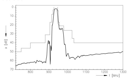
Transfer function (pass band, 25  $\pm$  5  $^{\circ}\text{C})$
